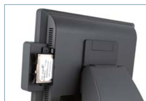
Slide in/out HDD replacement
